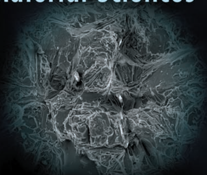
Ductile fracture taken on JSM-6610LV
