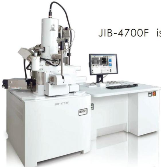
JIB-4700F is a new generation multi-beam FIB system.
